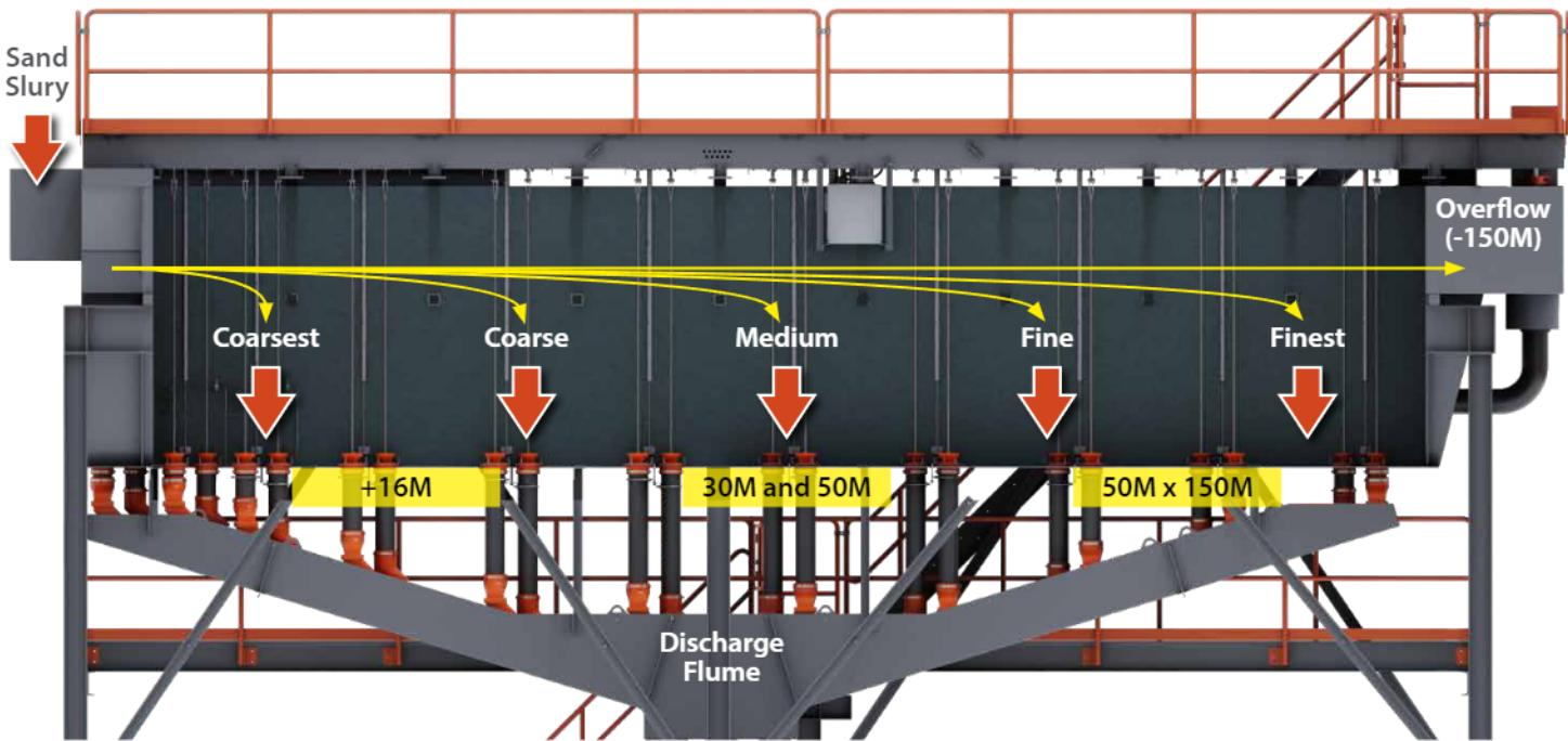
» Sand enters tank and flows along its length. Particles drop out as the velocity of the water slows and allows them to drop.
