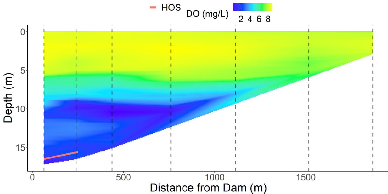
Figure 9: Lateral extent of hypolimnetic oxygenation in Calero Reservoir (September 3, 2021). The extent of the diffuser line is shown in red.
