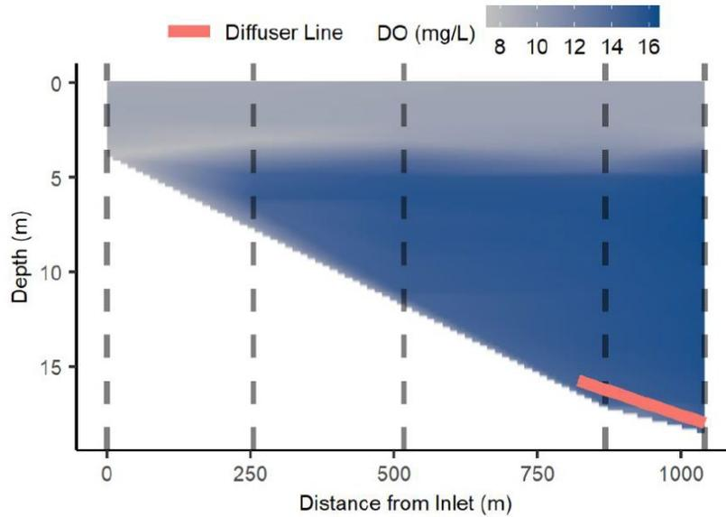
Figure 8: Lateral extent of hypolimnetic oxygenation in Almaden Reservoir (June 14, 2018). The extent of the diffuser line is shown in red.
