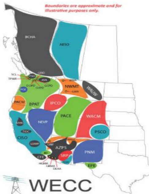
Figure 5 Balancing Authorities in the Western Interconnect
