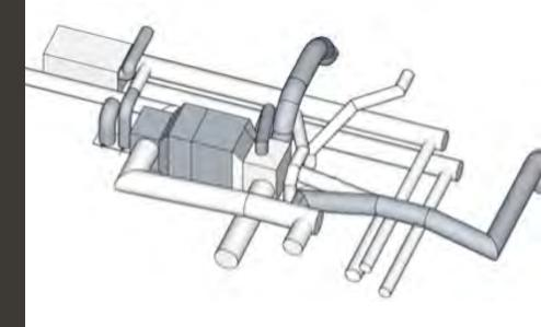
Santa Fe Ultra Series also offers the flexibility to be installed independently of the HVAC system. This allows for proper dehumidification throughout the home when ductless mini-split A/C systems are used.
