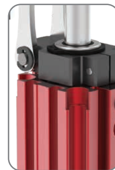
Integrated sensor slots in the body accommodates both, Ø4mm round and, 3x6mm T-slot style sensors.
