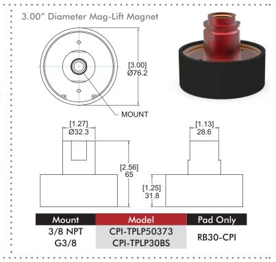
Note: The minimum air pressure required for the Mag-Lift to release parts is 25 psi. The suggested air pressure for normal operation is 35 psi. If part do not release immediately, increase the air pressure in 5 psi increments until the part releases. Do not exceed 60 psi. Air pressure should be measured at the inlet of the Mag-Lift to ensure effective operation.
