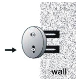
4. Put the base of bathroom accessory cover on the fixing blocks.
