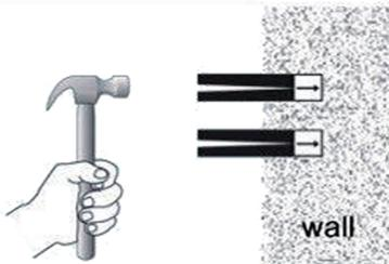
2. Put the expansion plugs into the wall by hammer.
