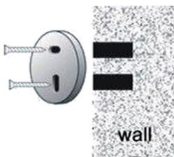
3. Put fixing block cover on the holes and fix firmly by expansion screws.
