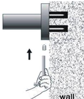
5. Screw grub screws into the base, make it against to the fixing block tight and firm.
