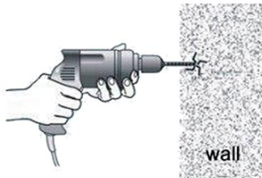
1. Put the fixing blocks (piece) over on the right place on the wall, and stay level, use marking pen through the holes of fixing block to mark out fixing spots on the wall. Then drill holes by electric hand drill with 6mm drilling bit on the spots.
