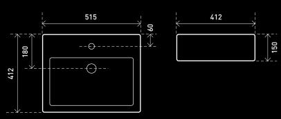
Measurement shown are in millimetres
