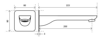
All measurements are in millimeters. For ceramic products, please allow +/- 5mm tolerance for manufacturing variance.
