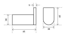
All measurements are in millimeters. For ceramic products, please allow +/- 5mm tolerance for manufacturing variance.
