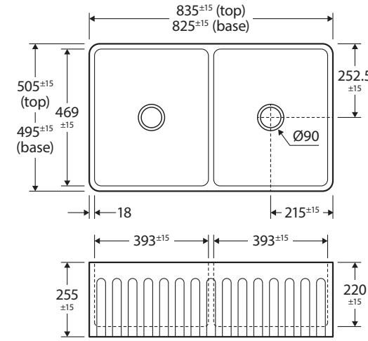
Please note: Butler sink measurements shown are a guide only. For installation, measurements must be taken from physical product received.
