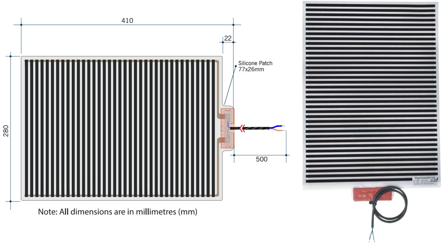
Note: All dimensions are in millimetres (mm)
