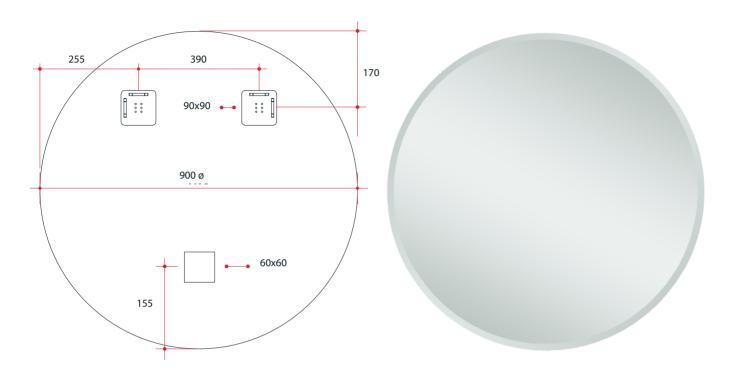
Note: All dimensions are in millimetres (mm)
