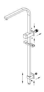
4.Adjust lower body position, and put diverter body and lower body on to the outlet adapter and the bracket, then tighten grub screws by Allen key.
