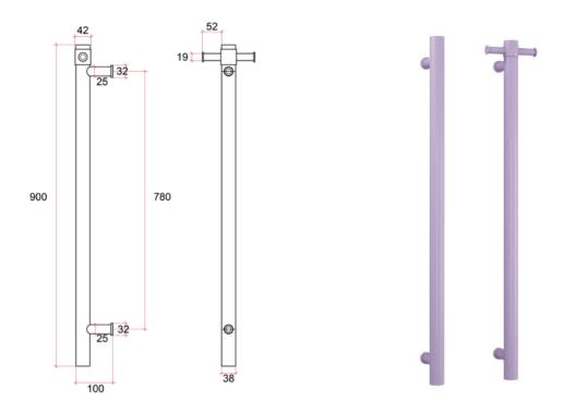
Note: All dimensions are in millimeters (mm)
