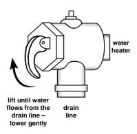
If water does not flow freely from the drain line when the lever is lifted, then the water heater must be checked. Phone Aquamax Service to arrange for an inspection.
