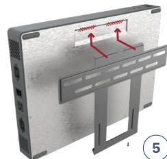
*Note: It is also possible to secure the mount to the underside of a table, bed, or cabinet. Please follow the above instructions, ensuring at least two screws are used to bite into the wood of the mounting surface. Then add one additional screw through the hole near the bottom hook on the mount (see image 6).*
