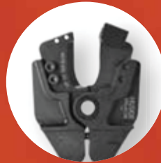
NEW EVS-ACSRJAW Cuts EHS Guy Wire up to 3/8" diameter & copper, aluminum up to 350 MCM, & ACSR up to 556 MCM.
