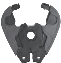
EVS-KJAW CRIMPS lugs & splices #8 to 500 MCM copper, #8 to 350 MCM aluminum, & H-Taps up to 4/0-4/0.
