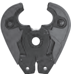
EVS-D3JAW CRIMPS lugs & splices #8 to 500 MCM copper, #8 to 350 MCM aluminum, & H-Taps up to 4/0-4/0.
