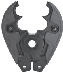
EVS-OJAW CRIMPS lugs & splices #8 to 500 MCM copper, #8 to 350 MCM aluminum, & H-Taps up to 4/0-4/0.
