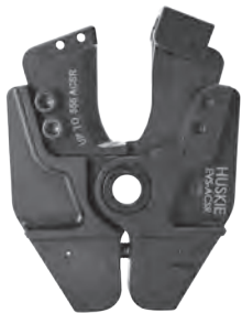
EVS-ACSRJAW REPLACEMENT BLADE: EVS-ASCR-8 CUTS EHS Guy Wire up to 3/8" diameter & copper, aluminum up to 350 MCM, & ACSR up to 556 MCM.
