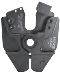
EVS-GWJAW REPLACEMENT BLADE: EVS-GW-8 CUTS EHS Guy Wire up to 1/2" diameter & copper, aluminum, & ACSR up to 4/0.
