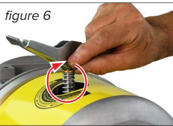
**STEP 2** Unlock and open the pinch roller. (*steps 2 and 3 above*)
