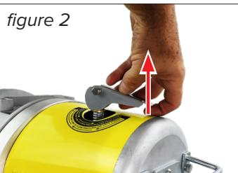
**STEP 2** Unlock the pinch roller lever by pulling it up. *figure 2*
