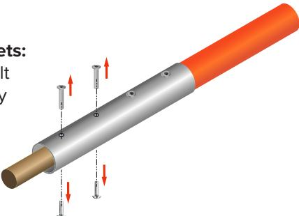
**2 Insert the Extension Pole:** Slide the extension pole into the base pole, ensuring the holes in the pole and steel tube are properly aligned.
