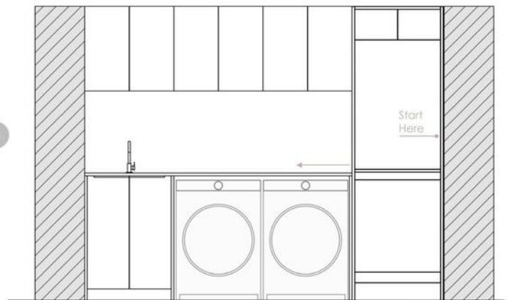
B. Wall To Wall - Start where you tall cabinet is. If there is no tall cabinet, start from either side. Tip - measure the total space first to ensure your cabinet will fit including fillers.
