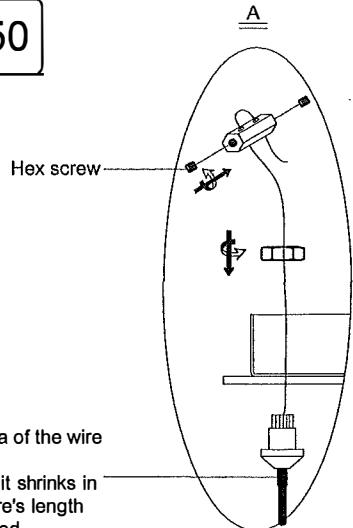
The dash area of the wire lock sleeve is flexible, when it shrinks in, the safety wire's length can be adjusted.
