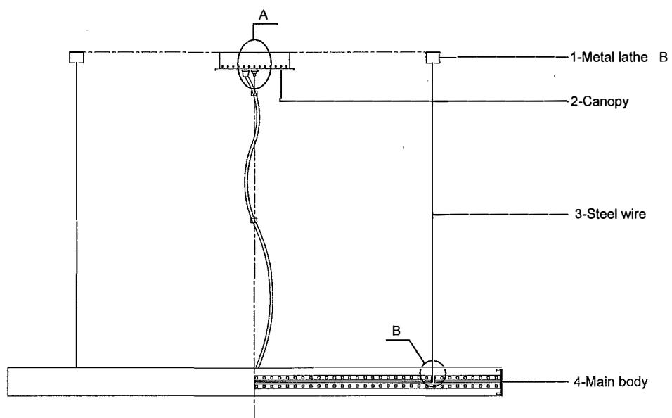
Could adjust steel wire's length when you use screw
