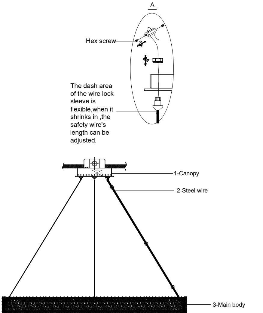
Could adjust steel wire's length when you use screw
