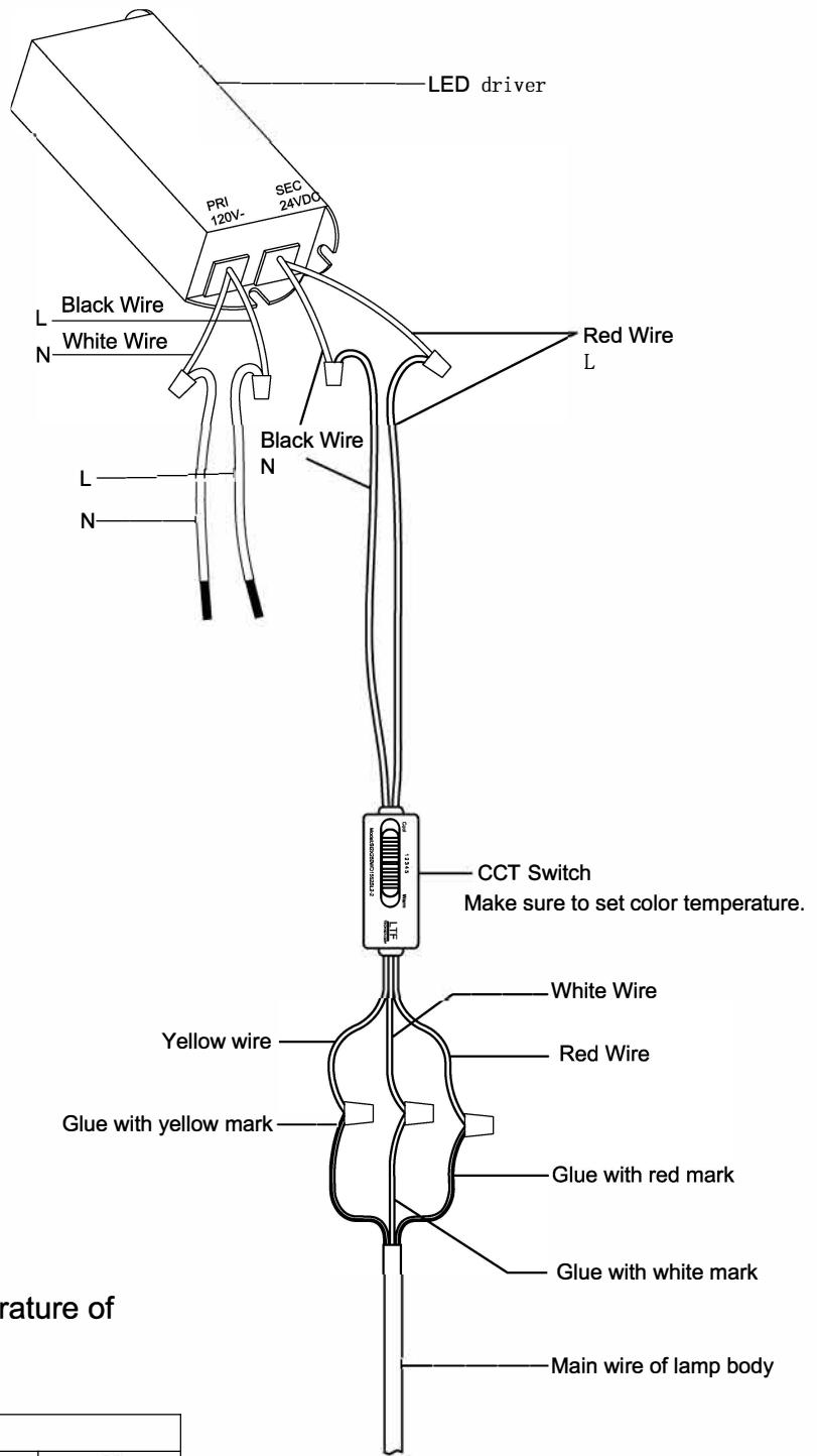
Note: Please adjust the color temperature of tape light before installing canopy!
