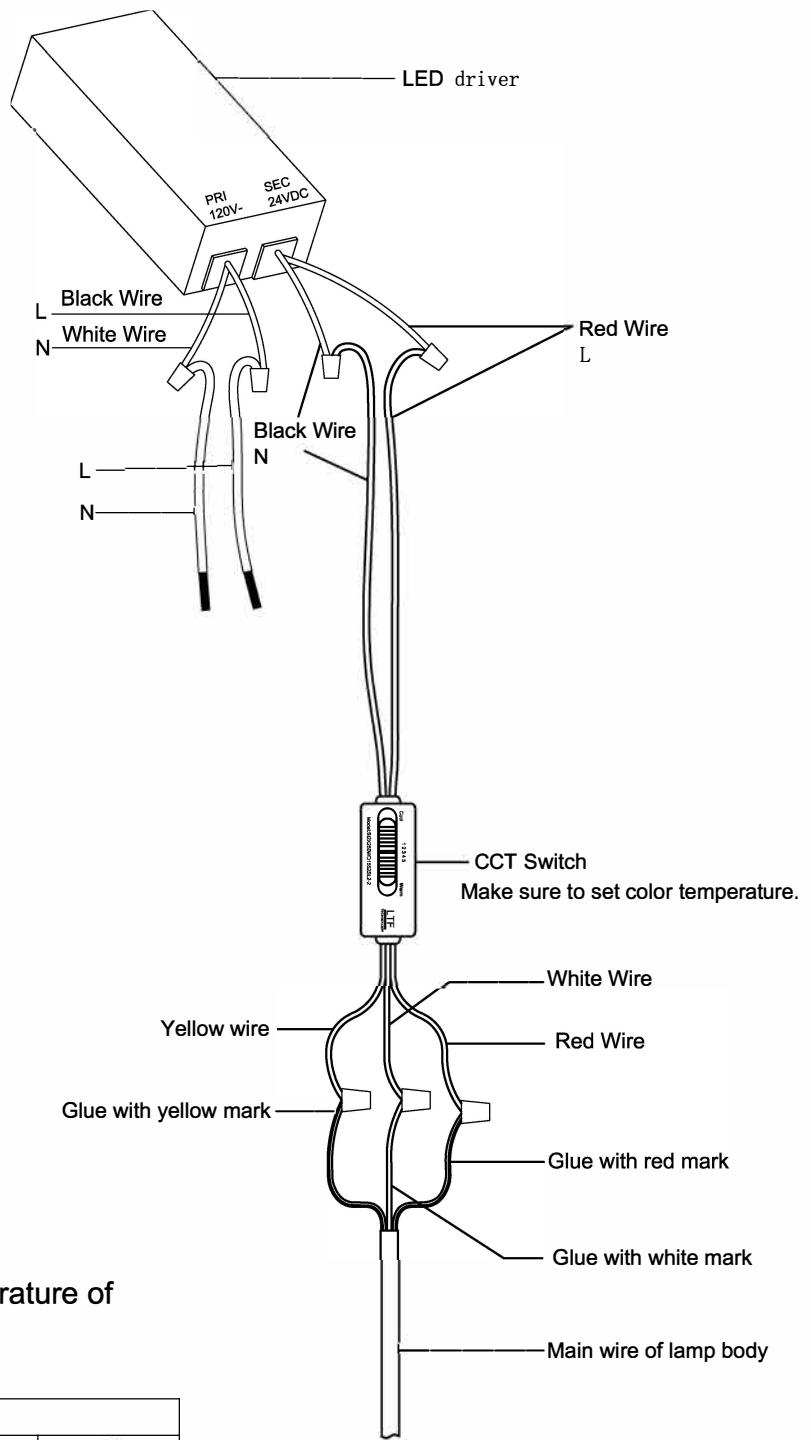
Note: Please adjust the color temperature of tape light before installing canopy!
