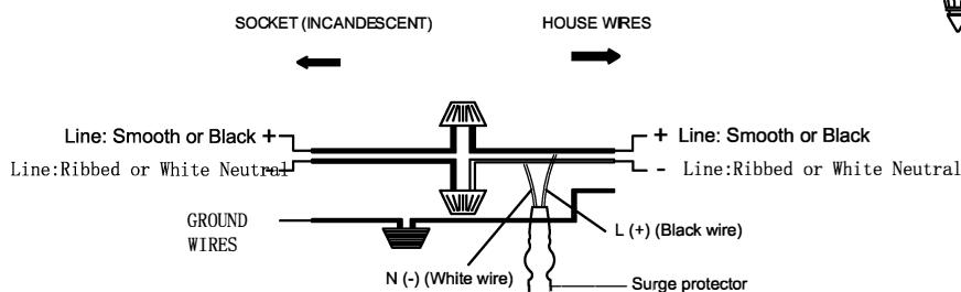
Note: It is recommended that each surge protector be connected to a maximum of 6 LED boards!
