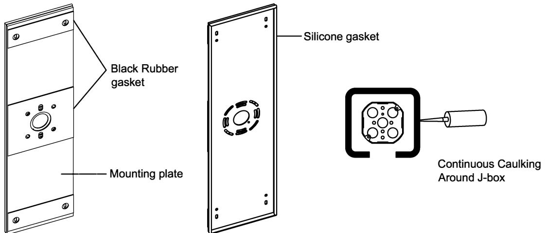
**3** Continuous caulking must be applied between wall and fixture frame by contractor.
