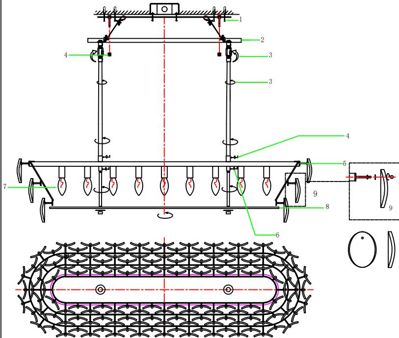
**STEP 3:** Refer to wiring diagram. With wire carefully threaded thru canopy, connect the black supply wire to the smooth fixture wire with wire connector, connect the white supply wire to the ribbed fixture wire with wire connector. Connect ground wire from fixture with supply ground wire.
