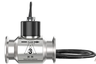
G3A Flow Meter, 2-Wire Magnetic Pickup with 10 ft. of Cable (Sine Wave Pulse)
