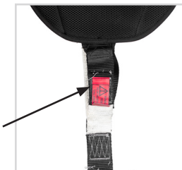
Red Exposed - Impact Indicator Broken - Remove From Service -
