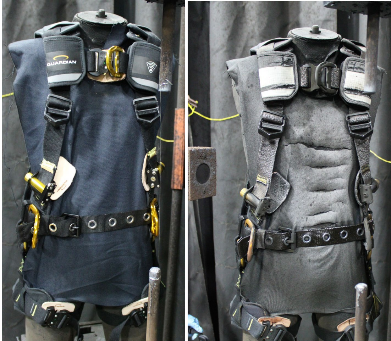
Figure 6.4 Sample before and after arc exposure, 24-00216A
