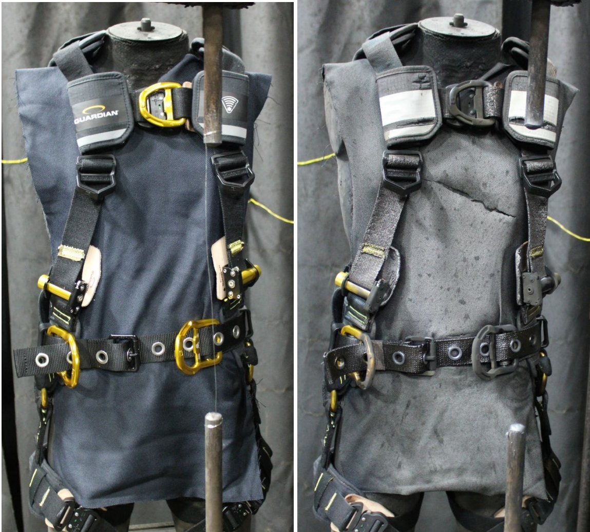
Figure 6.2: Sample before and after arc exposure, test 24-00213A.
