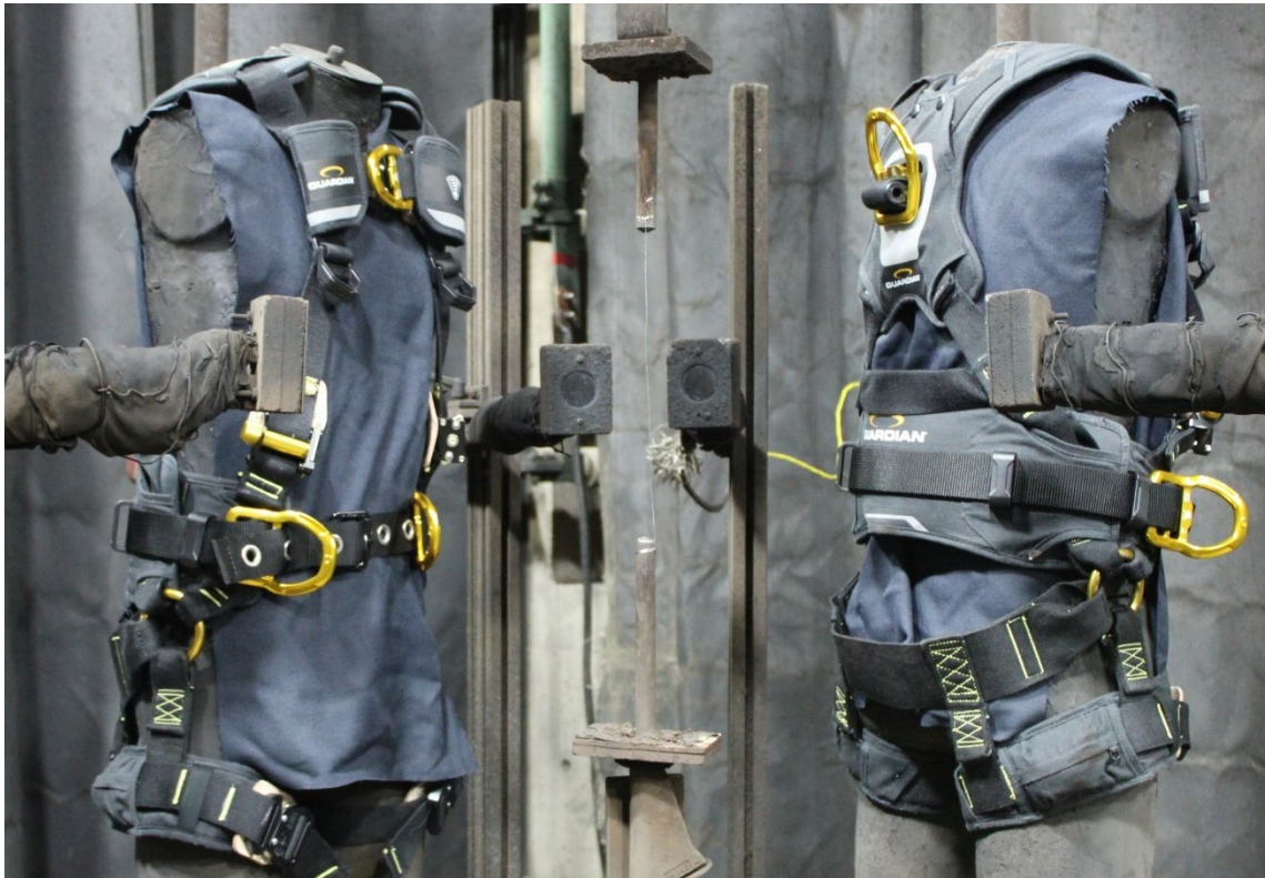
Figure 6.1: Sample set up before arc exposure.
