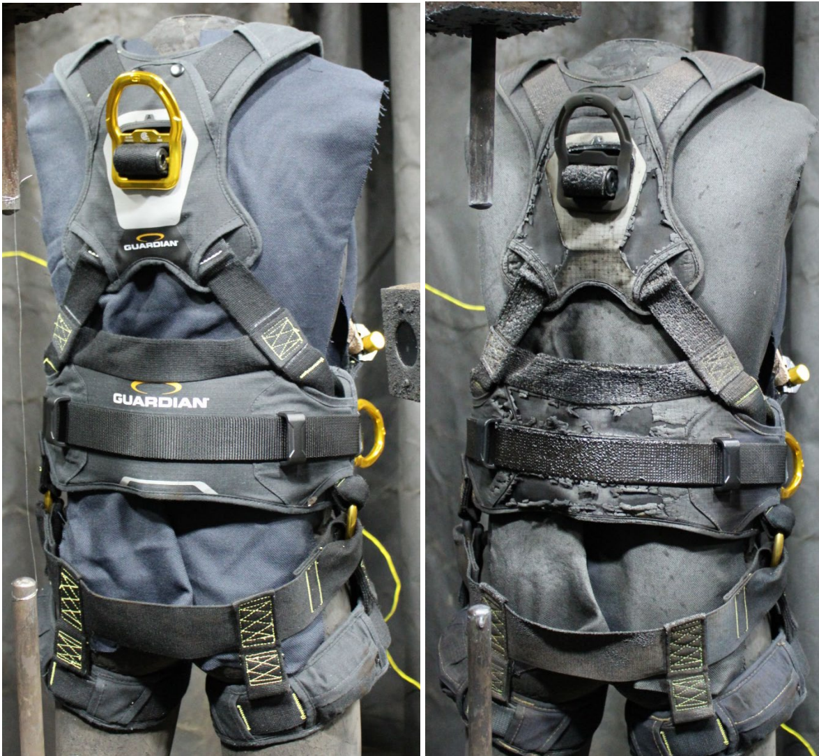
Figure 6.3: Sample before and after arc exposure, test 24-00213B.
