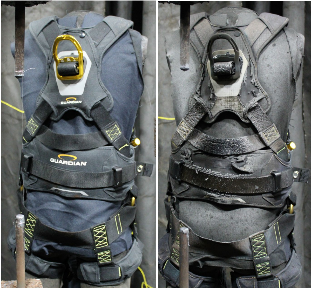
Figure 6.5: Sample before and after arc exposure, test 24-00216B
