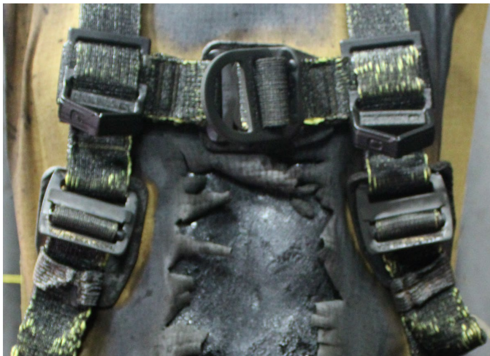
Figure 6.5: Webbing keepers and adjusters after the arc exposure, test 24-0836
