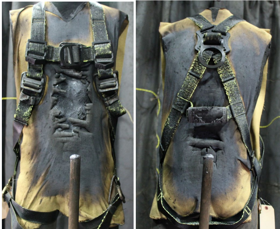
Figure 6.3: Sample after the arc exposure, test 24-0836, A: Left, B: Right.
