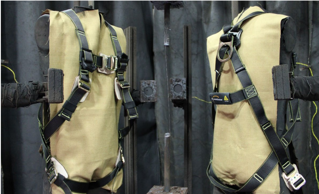
Figure 6.1: Sample set up before the arc exposure,
