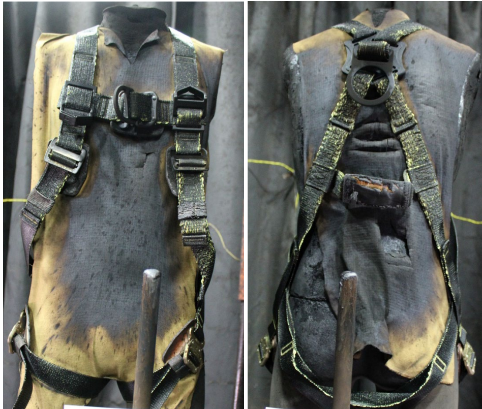
Figure 6.2: Sample after the arc exposure, test 24-0831, A: Left, B: Right.
