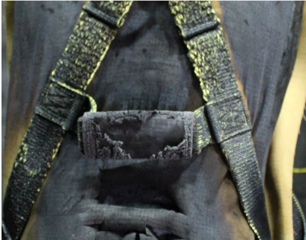
Figure 6.4: Label pouch after the arc exposure, test 24-0836
