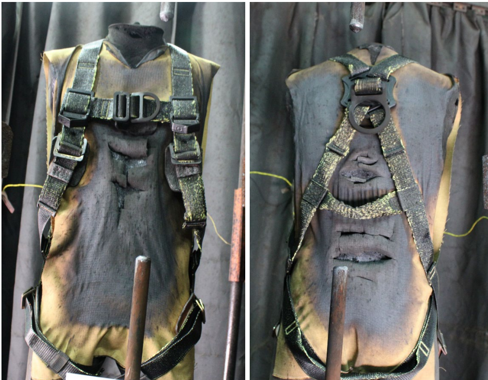
Figure 6.3: Sample after the arc exposure, test 24-0841, A: Left, B: Right.
