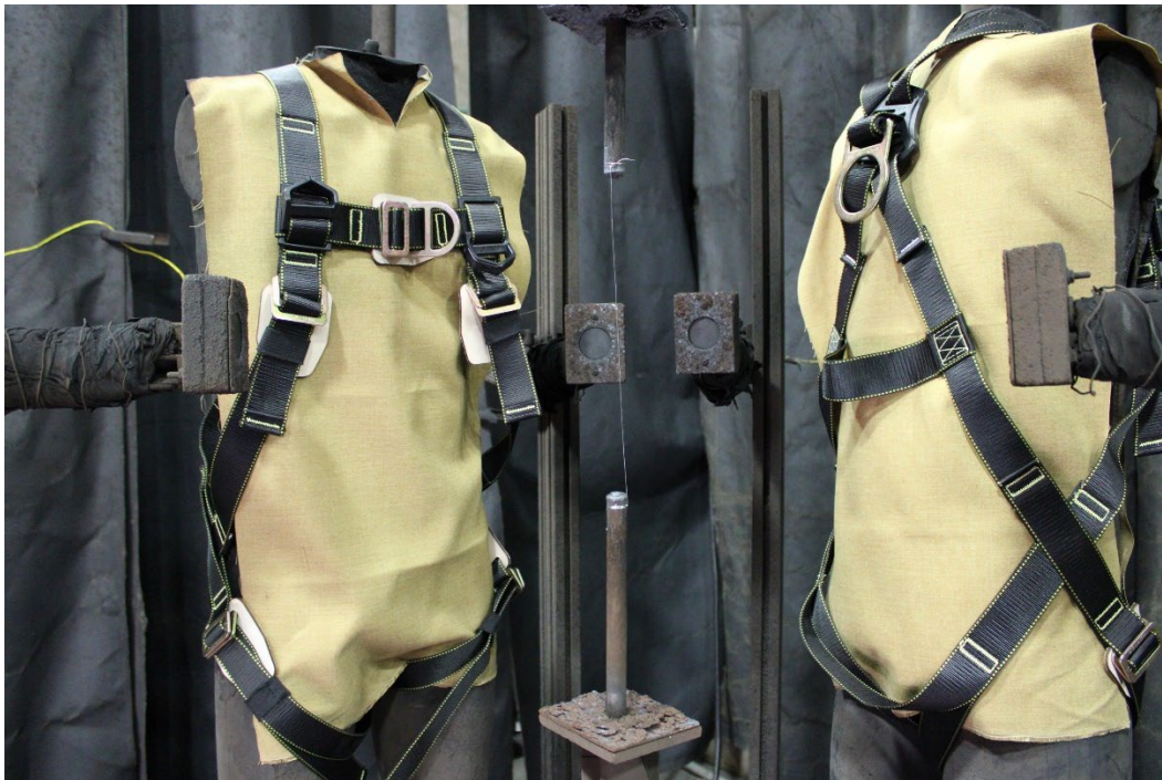
Figure 6.1: Sample set up before the arc exposure.
