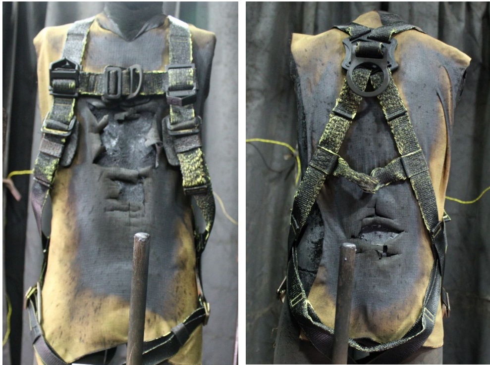
Figure 6.2: Sample after the arc exposure, test 24-0837, A: Left, B: Right.
