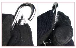
Open the carabiner gate by unscrewing the screw collar counterclockwise and insert the tether attachment point (D-Ring, Key Ring, etc.) of the tool onto the carabiner. Once in place be sure to screw the collar clockwise until tight into place preventing the carabiner from inadvertently opening.
