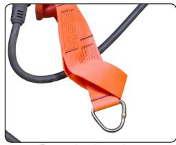
To create the tether attachment point, slide the D-Ring through the loop. Position the Cinch Loop to a location that won't impede the usefulness of the tool and then pull and tighten by hand.
