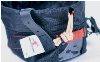
2. Excessive wear to the rope at the tether loop cinch point.
