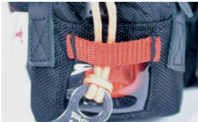
3. Excessive wear to the fabric, stitching, tensioning strap, and belt components.
