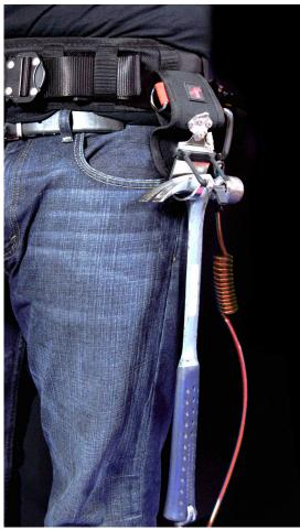
Attach bungee or coil style lanyards (Max Tether Length 4 ft) to D-Rings or use one of many our many retractable tool lanyards.
