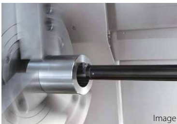
KAV-G20-10D / KAVH20-SCLCR09 CCMT3251PP Overhang length: 140 mm (7D) / 200 mm (10D) Workpiece: 4137
