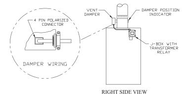
FIGURE 6.2: VENT DAMPER INSTALLATION DETAILS
