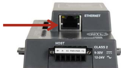
Figure 3 - Ethernet Connection on the ProtoNode
