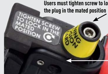
Zone 2/Division 2 DR30 receptacles feature a standard screw-type locking pawl. This required feature allows the user to lock the plug to the receptacle by tightening a screw on the pawl.
