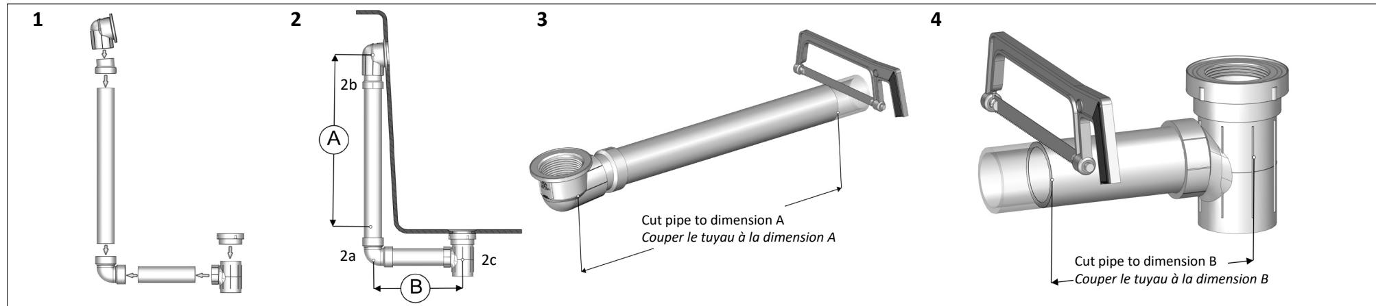
Step 2a,2b,2c: Dry fit pipe approximately 0.75" (2 cm) into elbow 2a, overflow angle adapter 2b & drain Tee 2c. Measure pipe according to dimensions A & B.
