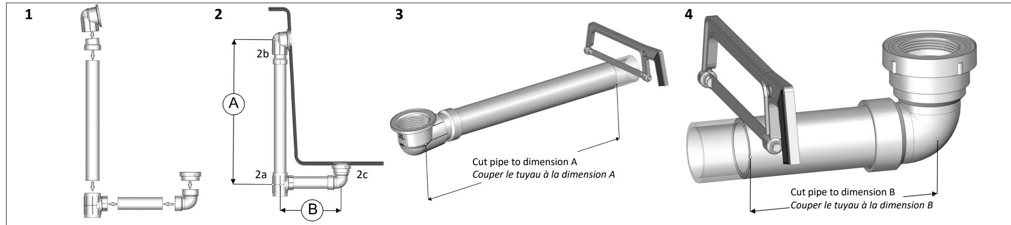
Step 2a,2b,2c: Dry fit pipe approximately 0.75" (2 cm) into Tee 2a, overflow angle adapter 2b & drain Elbow 2c. Measure pipe according to dimensions A & B.
