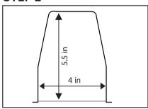
This 5/6" retrofit kit must be installed in a can with dimensions described within above diagram.
