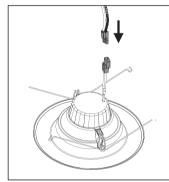
Plug the female connector of the RETROFIT KIT onto the male connector of the QUICK CONNECT ADAPTER.
