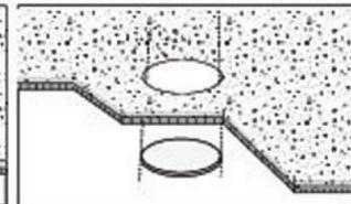
Cut a hole in the ceiling according to the dimensions listed below. Before you begin, ensure that the hole you are going to be cutting does not interfere with studs, piping, electrical or other building structures.
