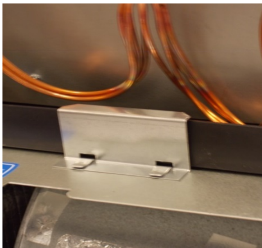
Figure 6-Coil hold down clip installed
