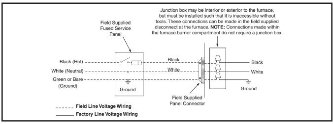
Figure 22. Line Voltage Field Wiring
