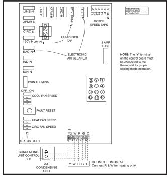
Figure 24. Emerson Low Voltage Field, Fourwire Heating/Cooling Applications
