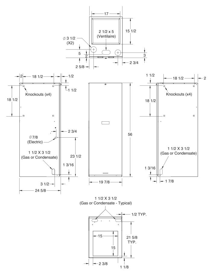
Figure 29. Top Return Cabinets (Without Coil Box)
