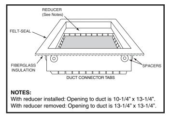
Figure 9. Duct Connector
