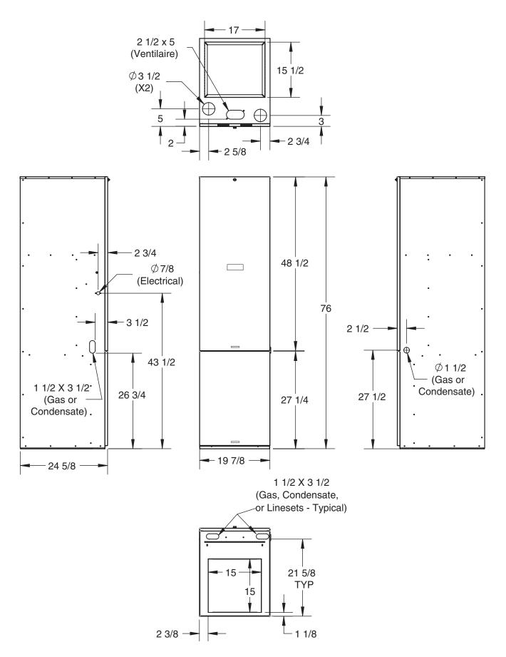
Figure 31. Top Return Cabinets (With Coil Box) (return cabinets ending in 'ACM)
