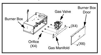
Figure 21. Orifice Removal
