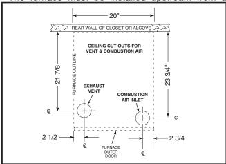
Figure 11. Ceiling Cut-Out Dimensions
