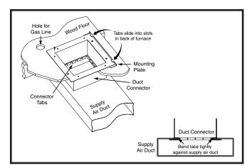
Figure 12. Finger Tabbed Duct Connector
