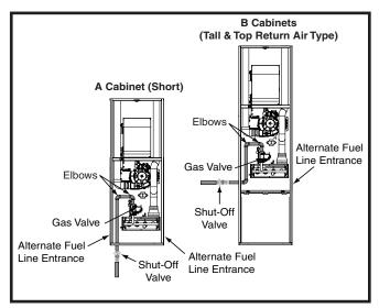
Figure 19. Typical Gas Connections
