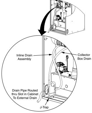
Figure 18. Condensate Drainage
