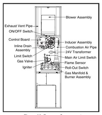
Figure 25. Furnace Components
