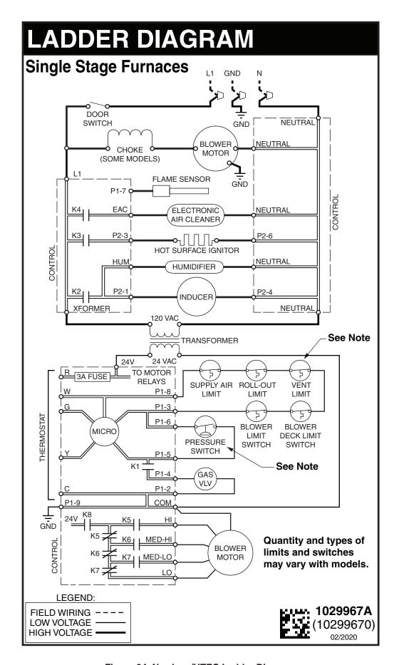
Figure 34. Nordyne/UTEC Ladder Diagram
