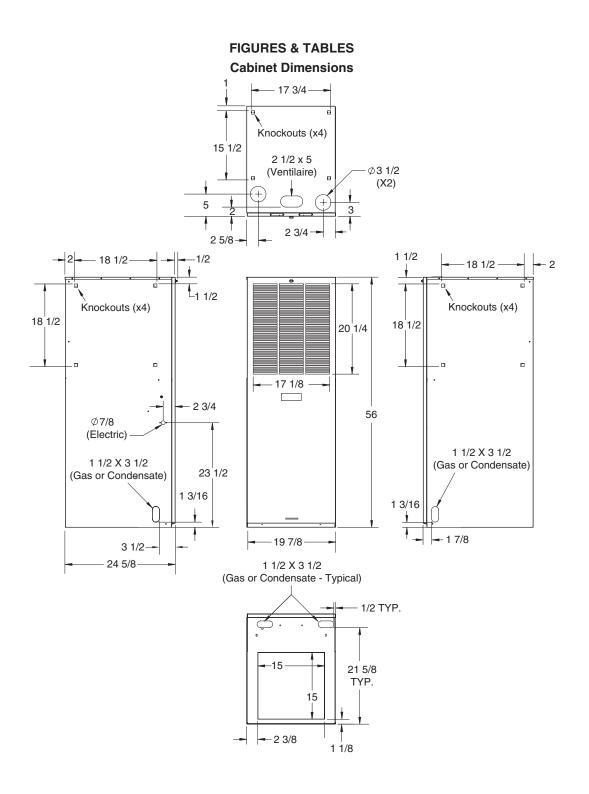
Figure 26. Front Return Cabinets (Without Coil Box)
