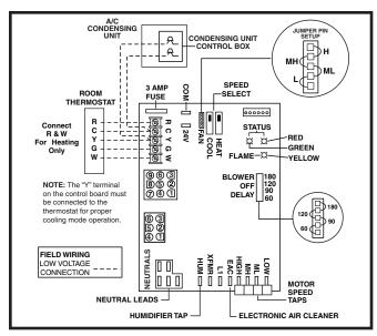
Figure 23. Nordyne/UTEC Low Voltage Field, Fourwire Heating/Cooling Applications
