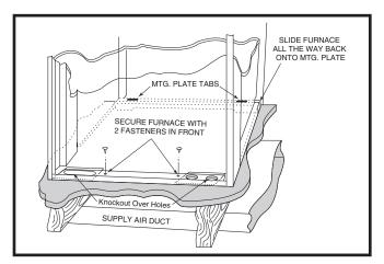
Figure 17. Cabinet Furnace on Supply Air Duct
