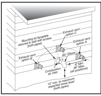
Figure 1. Inlet & Exhaust Pipe Clearances
