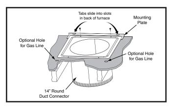
Figure 16. Round Duct Connector
