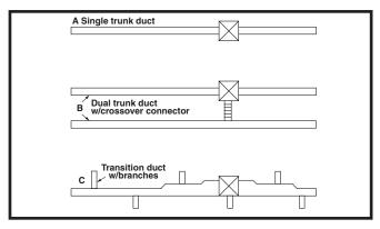
Figure 7. Typical Supply Duct Systems
