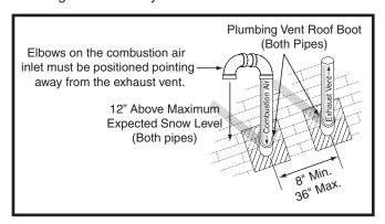
**Figure 4. Vertical Vent Termination**
