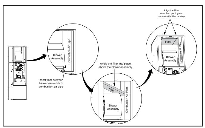
Figure 8. Filter Installation
