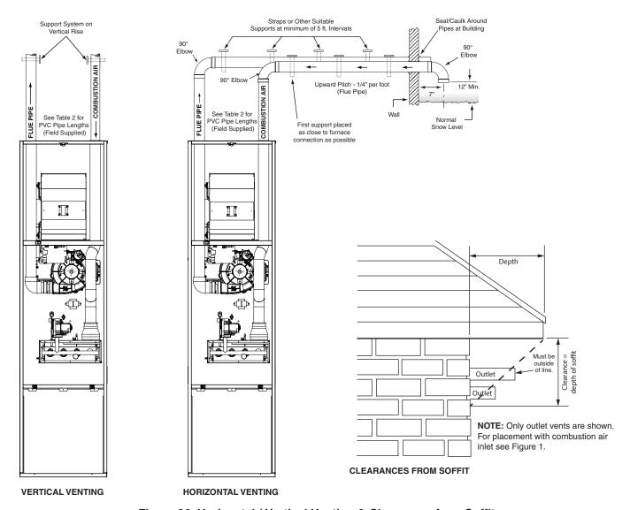
Figure 36. Horizontal / Vertical Venting & Clearances from Soffit
