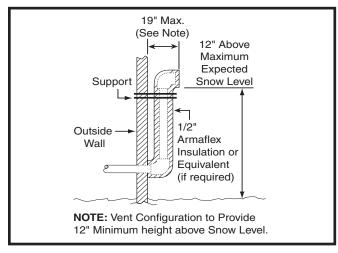
Figure 3. Alternate Horizontal Vent Installation
