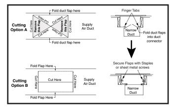
Figure 13. Screw-Down Duct Connector
