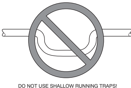
Fig. 10 – Insufficient Condensate Trap
