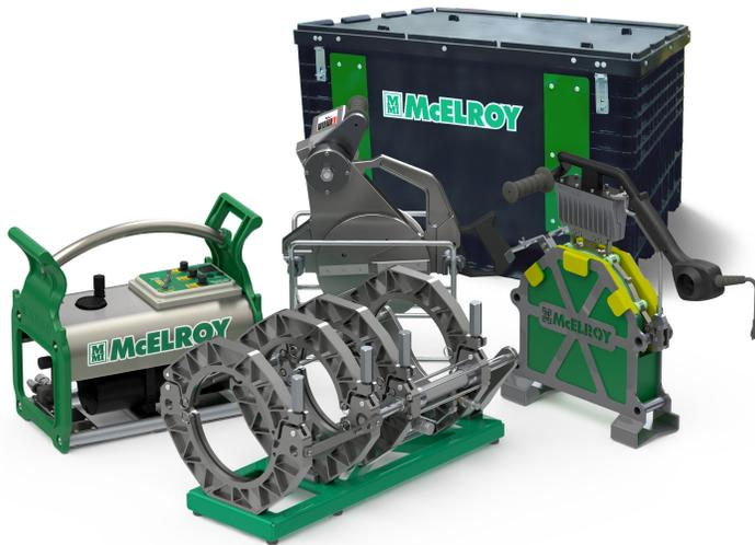
The Acrobat™ 250 has a compact design for easy maneuvering in tight work spaces and is capable of fusing pipe on the ground, vertically and overhead. To further reduce its footprint, the carriage can be configured from 4 to 3 jaws without tools. A single-size insert design can accommodate a variety of pipe sizes, and its narrow jaws allow fusions to most flanges and fittings.
